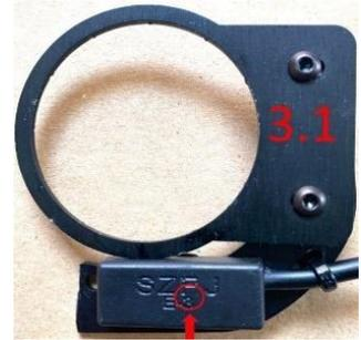
**Warning:** The area where the sensor detects movement is at the height of the "F" of the "SZFJ" script (photo 3.1) this letter must be placed as close as possible to the axis, any reversal of position of one of the elements will cause a malfunction.
