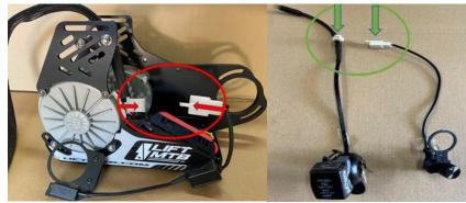
For models before August 2020 the operation remains the same, simply the wiring changes for this it will be necessary to connect the connector of the sensor in series on the trigger connector (yellow arrows on the photo).
