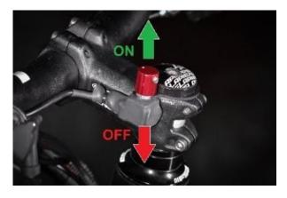
**WARNING:** When installing, do not bend the wires , and do not twist them at the end of the knob, do not overexpose the knob to the water.
