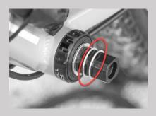
Finally tighten the left crank, respecting the steps and the torque as shown on the picture opposite (from 1 to 3):
